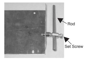
Figure 8 - Damper Adjustment
