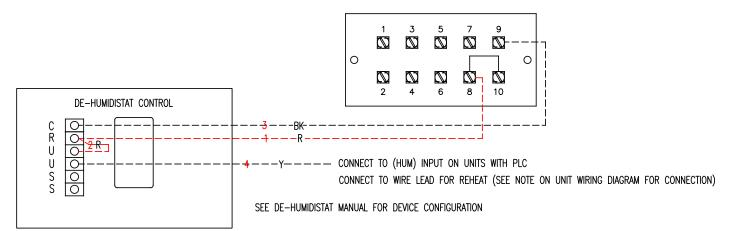
Figure 5a - Humidity Control Wiring Detail - Heat Pumps
