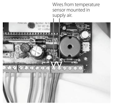
Figure 6 - Temperature Sensor Wires
