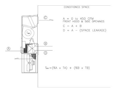
Figure 9 - Damper Air Path
