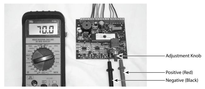
Figure 7 - Desired Temperature Set Point
